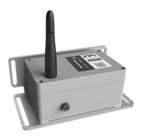
The Dynamic Displacement Sensor (DDS) is a wireless device that remotely monitors the dynamic displacement and the frequencies of infrastructures.
