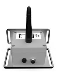
The triaxial Vibrometer is able to measure the velocity of the point where it is installed, providing complete frequency and amplitude analysis of vibrations. With the use of Vibrometer devices it is possible to highlight any seismic vibrations, mainly induced by external factors, and monitor their risks. Battery power supply and LoRaWAN wireless transmission. The acquisition modes can be set by the user via the web interface provided in the service.
