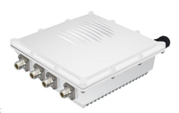
The device is Outdoor IP67 and is powered by PoE; optionally it can be powered by battery, with solar panel. The SHM Gateway is equipped with LoRa, LTE, GPS and high gain Wi-Fi antennas. Thanks to the dual LTE antennas, increased cellular coverage is possible. The device also implements a Wi-Fi hotspot and a built in GPS for very precise synchronization and geolocation of the product. It is very easy to set up thanks to the automatic APN and the included PoE adapter.
